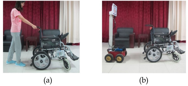
Fig. 13. Pushing a wheelchair. (a) A local user is pushing a wheelchair. (b) A remote user is remotely "pushing" the same wheelchair via a telepresence robot.
